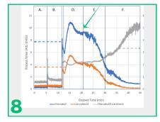
Identify signal equilibrate during full flow; identify **end point** by Cannabinoid and Chlorophyll signals stabilizing
