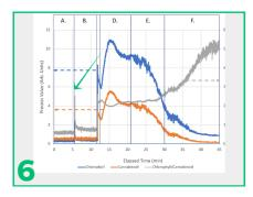
Observe no signal or noisy signal from reverberations during initial startup
