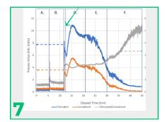
Identify signal spiking then dropping after initial fluid flow
